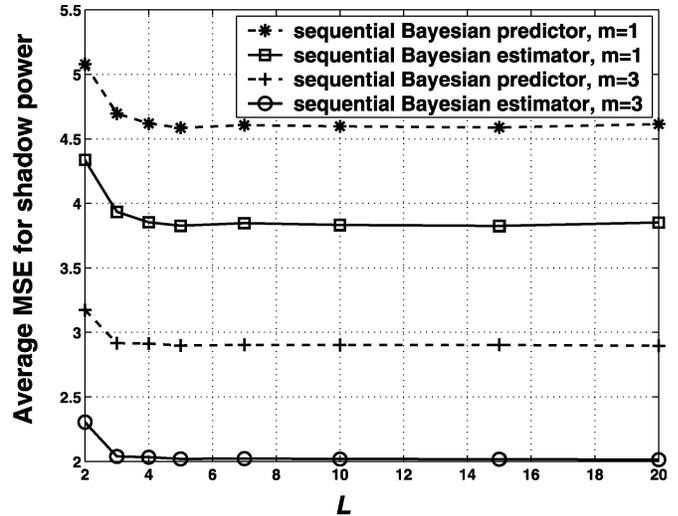
Fig. 3. Average MSEs for the sequential Bayesian estimator and predictor of the shadow powers as a function of the quadrature order  $L$ , for  $K = 200$  and  $m \in \{1, 3\}$ .
