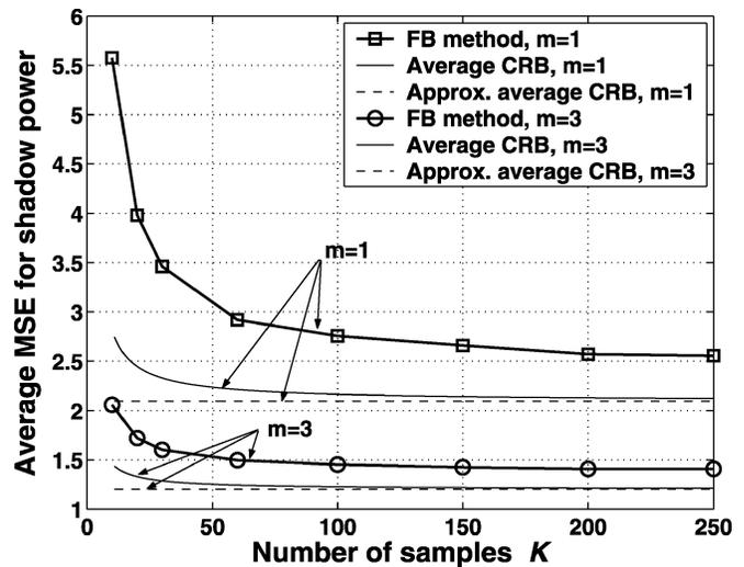
Fig. 4. Average MSEs and corresponding CRBs for the FB estimates of the shadow powers as functions of  $K$ , assuming known model parameters and  $m \in \{1, 3\}$ .
