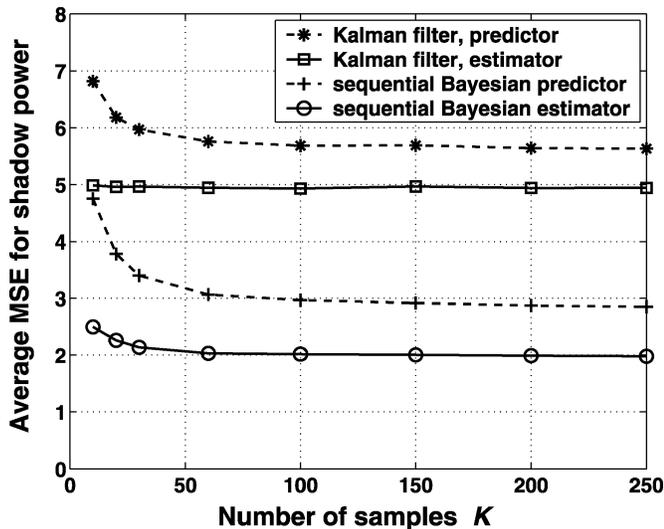
Fig. 2. Average MSEs for the sequential Bayesian and Kalman-filter-based estimators and predictors of the shadow powers as functions of  $K$ , assuming known model parameters and  $m = 3$ .
