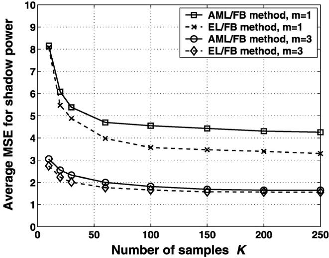
Fig. 5. Average MSEs for the AML/FB and EL/FB shadow-power estimators as functions of  $K$  for  $m \in \{1, 3\}$ .
