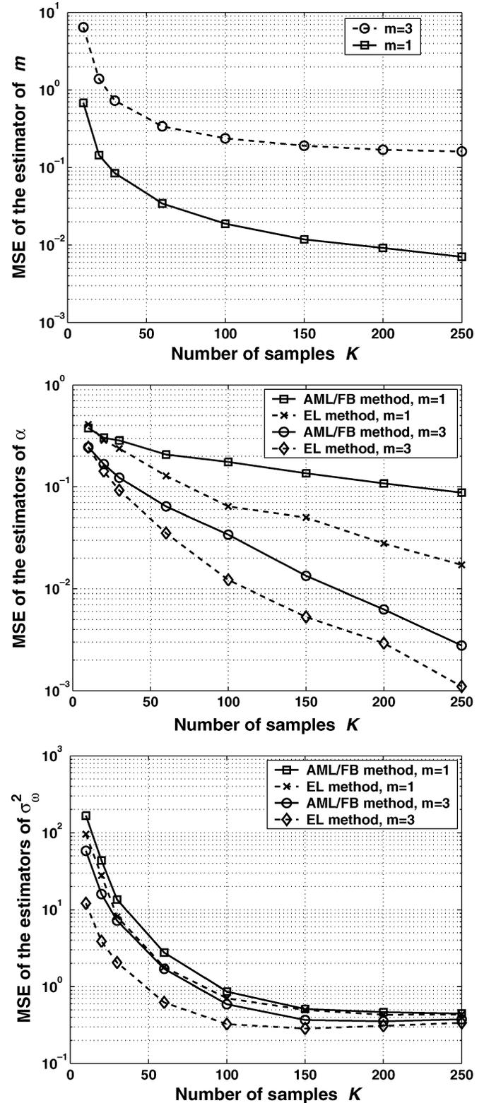
Fig. 6. MSEs for the AML/FB estimates of the model parameters ( $m$ ,  $\alpha$ , and  $\sigma_w^2$ , respectively) as functions of  $K$ , for  $m \in \{1, 3\}$ .
