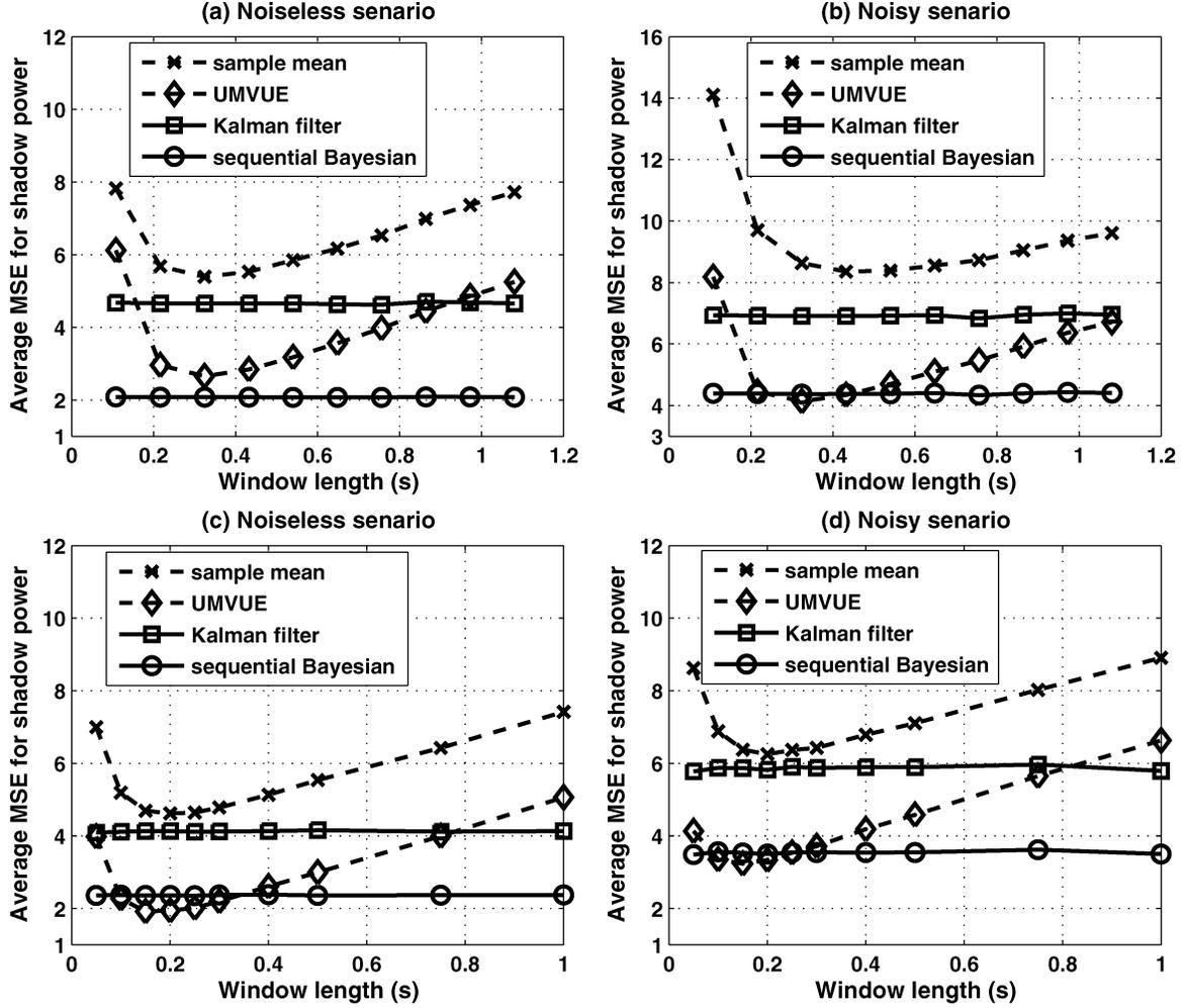
Fig. 7. Average MSEs for the sequential Bayesian, Kalman-filter, and window-based shadow-power estimators as functions of the window length, assuming correlated Ricean fading with (a)  $\sigma^2 = 0$  and  $T = 54$  ms, (b)  $\sigma^2 = 0.2$  and  $T = 54$  ms, (c)  $\sigma^2 = 0$  and  $T = 5$  ms, and (d)  $\sigma^2 = 0.2$  and  $T = 5$  ms.
