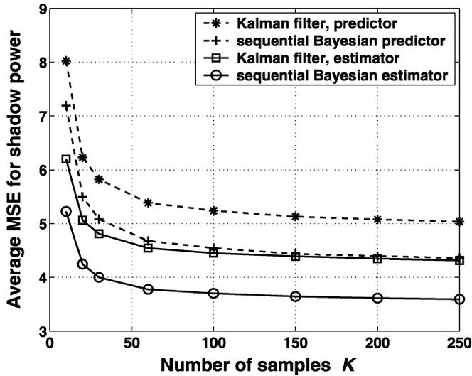
Fig. 1. Average MSEs for the sequential Bayesian and Kalman-filter-based estimators and predictors of the shadow powers as functions of  $K$ , assuming known model parameters and  $m = 1$  (Rayleigh fading).
